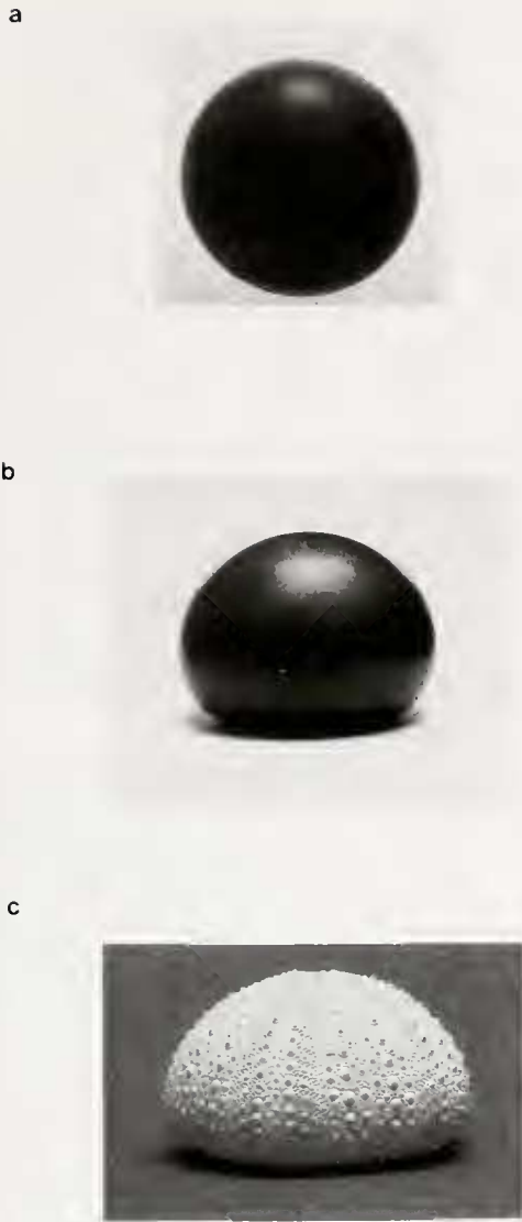
Figure 1. (a) A balloon filled with water in water; (b) a balloon filled with water in air; and (c) an urchin test. Note the similarity of shape between the (b) and (c). The difference in shape between (a) and (b) illustrates the importance of self-weight forces. There are no self-weight forces on a water-filled balloon in water since the water inside and outside are equally dense. In urchins, the internal volume also has no effective weight; thus the downward forces result only from the underwater weight of the calcite or the pull of tube feet. The weight forces are balanced by internal pressure resulting from tension in the membrane. None of these structures are pneus because they are not air-filled, but (a) and (b) certainly, and (c) possibly, form their shape as a result of forces analogous to those in a pneu, including internal pressurization.
